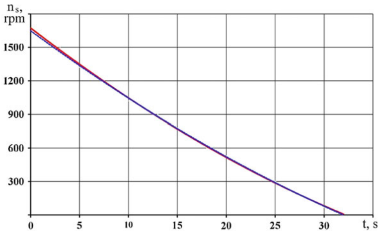
Fig. 5 Approximated dependences of the stand dynamometer rotation speed on the car runout time: — for NPT; — for BL-85 175/70R13 pneumatic tires
