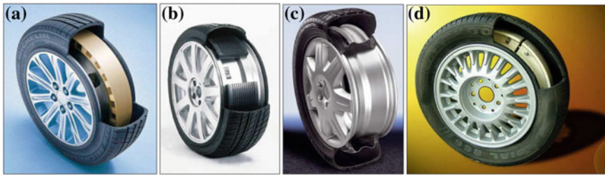
Fig. 1 Automobile high-safety wheels with inner emergency supporting bodies: a Michelin PAX; b Pirelli PAX; c Continental CSR; d Hankook with support ring Rodgard
